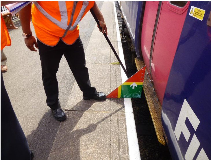
Platform clearances. Checking the stepping distance between a class 150 train and a platform on the West Somerset Railway.
